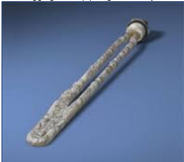
Figure 44: Lime Scale Build Up
